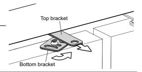
3. Fit a lock through the brackets to secure the doors. When the lock is removed, slide and rotate the brackets back into the cabinet.
