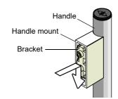
4. Fit and screw the bracket/s back onto the door. Ensure the catches are pointing up as pictured.
