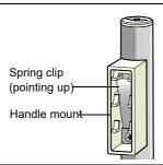
3. Locate BOTH handle mounts simultaneously onto both door brackets. Then push the handle down onto the brackets, until the handle locks into place.
