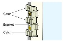
5. Refit the door gasket by clipping it back into place on the inside of the door frame. If the gasket is out of shape after refitting it, a hair drier can be used to heat and reshape it.
