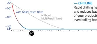
Rapid chilling halts the deterioration of foods, stops oxidation and reduces bacterial growth. MultiFresh® Next brings the core of your products to +3°C from any starting temperature, even boiling hot, maintaining food properties.
