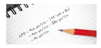
In the above example, the conductivity of the decarbonised water is below 100 µs/cm, which means that the water is suitable for washing glassware. Partial demineralisation is therefore sufficient.
