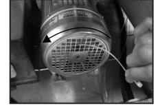
▶ If not, interchange two of the three phase on the feed cable.
