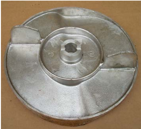
E6414 under side of the abrasive disk showing the drive slot.
