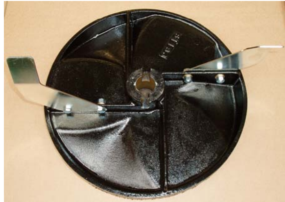
E6128 under side of the abrasive disk showing the drive slot.
