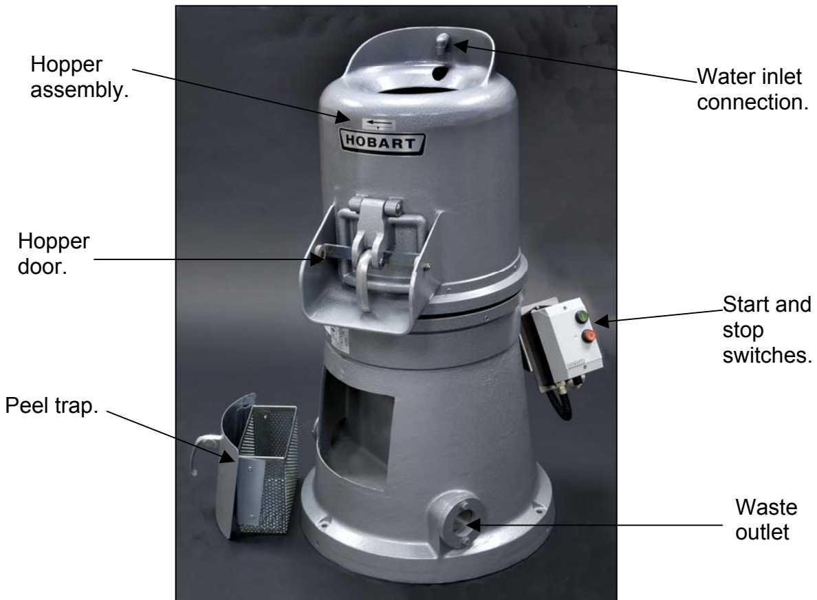
FIGURE 2. E6128 COMPONENT IDENTIFICATION.
