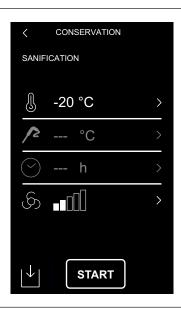
The arrows on top allows moving among the various phases fo the sanification to visualize/adjust setpoints. After selecting the function, a screen containing the presets is displayed, which can be adjusted.
