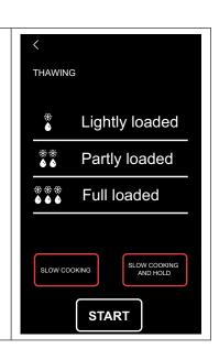
At the end of the **THAWING** cycle, the buzzer ringsn and **STORAGE** starts with endless duration.
