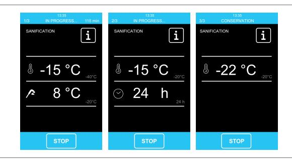
During chilling, the appliance displays the temperature detected by the core probe, the chamber temperature and the time elapsed since chilling has started.
