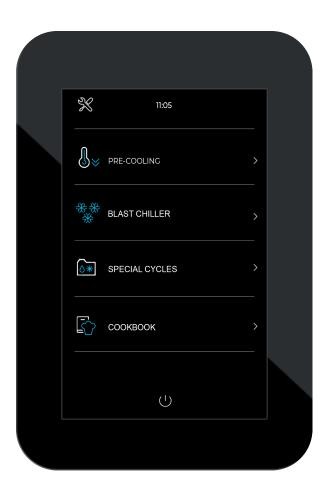
In case of power interruption during "STAND-BY" or "ON" status, when power will be restored the control panel will resume the current status before the interruption.
