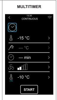
Cycle is started by pushing the key; it ends only when all timers are elapsed; after this, the STORAGE phase begins
