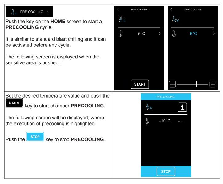
Once the desired temperature is reached, the buzzer rings and the cycle continues by keeping the reached chamber temperature until the stop key.
