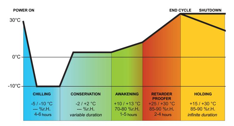
An automatic retarding-proofing cycle is composed of 5 different phases with different temperatures, relative humidities, fan speeds and durations. All these phases are automatically carried out one after the other, as per following details:
