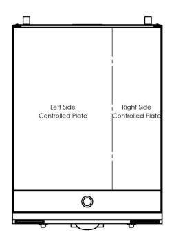
The hotplate is designed in such a way that heat pools in the centre of the hotplate, with the front and rear corners being comparatively cooler. This allows the user to balance the cooking times of multiple products/foods that require different temperatures or times to cook.
