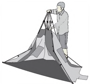
Standing close to the central hub, lift the top of the hub to head height.
