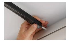
7. Turn the knurled knob and lock Curved Roof Rafter in place.
