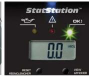
LCD STATSTATION<sup>TM</sup> Displays total power used, total unit hours, and maintenance reminders Model #020654 (#2205)
