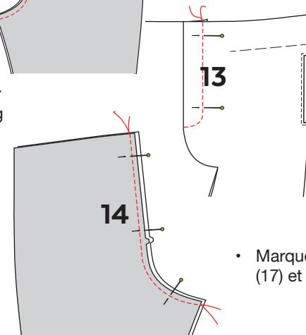
Diagram 14: Pinning the back pieces at the crotch seam.
