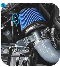
Now that everything is in assembled, lock the location in place by tightening the 2 x M5\*10mm hex flange screws which you pre-assembled in STEP 2 using a 7mm socket or spanner, highlighted in Figure 3c.
