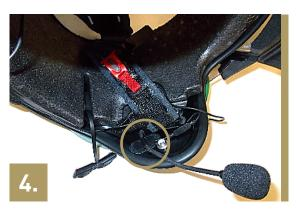
Place the microphone base under the chinstrap between EPS and shell. Use the additional microphone support included by positioning it as the image.
