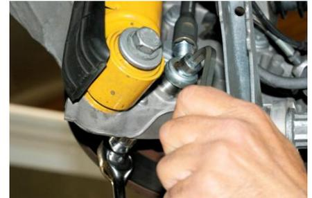
8. Tighten M10x55mm bolt and factory nut using 8mm hex key wrench and 16 mm deep socket. Torque to 45 Nm (33 ft lbs.).
