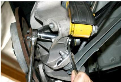
5. Unbolt end link from trailing arm using a 16mm deep socket and 16mm or 5/8 inch thin open end wrench, then remove end link. Repeat for other side.
