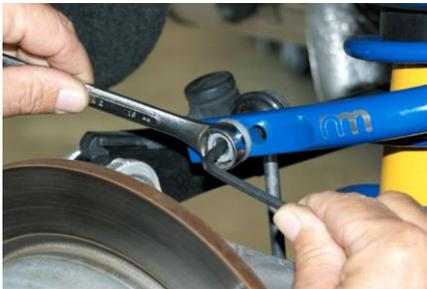
4. Unbolt nut from rear anti-sway bar to end link using a 16mm wrench and 5mm hex key wrench. Repeat for other side.
