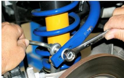
7. Tighten bolt using 8mm hex key wrench and 16mm wrench. Torque to 45 Nm (33 ft. lbs.)
