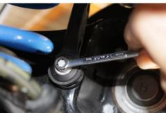
Back out lower end-link mounting bolt about a using an E10 Torx or 5/16" wrench or socket. Pull down on anti-roll bar arm due to bushing pre-load and then pull out upper endlink stud from bar. Repeat for other side.
