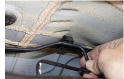
10. Brake lines will unclip from their NOTE: support mounts on the uni-body.
