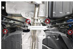
Remove the (4) sub-frame mounting bolts using E14 Torx or 7/16" socket. Supporting sub-frame not required.
