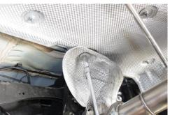
Unbolt [1] 10mm hex nut from exhaust heat 8. shield that connects from sub-frame to uni-
