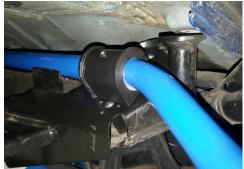
Apply supplied grease to inside of supplied urethane bushings and install on NM anti-roll
