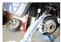
Install NM anti-roll bar in reverse of removal of original bar being careful getting around brake lines. HINT: Leave plastic wrap on bar to protect finish of bar during installation through sub-frame then remove.
