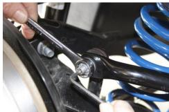
Remove upper end-link nut from anti-roll bar by securing stud with T30 Torx or 4mm hex key wrench and loosening nut with 16mm wrench. Repeat for other side.
