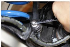
Attach upper end-links to NM anti-roll bar using original nuts. Torque to 48Nm (35 ftlbs). Then tighten lower end-link bolt. Torque to 34Nm (25 ft.-lbs.). See adjustment chart for hole position information. NOTE: NM Eng. Rear Sway Bar Link Kit recommended.
