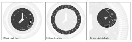
Clasp the outer face of the dial and rotate it clockwise. The internal ratchet will emit a buzzing sound that is normal. Stop rotating when the correct time is reached. If you overshoot, then continue turning clockwise until the correct time is reached. 12 hour indication is displayed by an hour hand and a minute hand on the inner dial. 24 hour indication is displayed on the outer dial. The timer depicted indicates 7 on the inner dial and 19 on the outer dial. Hence the time is set to 7:00pm.
