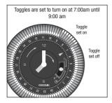
The example to the left has eight of the toggles on the outside position. The timer is set for a time of 7:00am. The toggles from 7:00am to 9:00am are in the outer position. These will activate the switch when they align with the 24 hour clock indicator. At 7:00am, the chlorinator and pump will turn on and at 9:00am, they will turn off.
