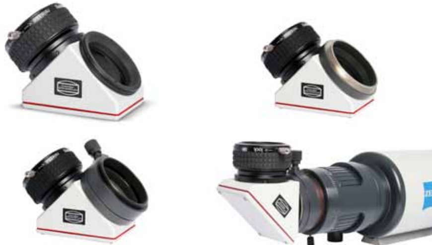
Adaptation of the M68 star diagonal. Top left: The exposed M68 thread. Top right: With M68 / S68 Zeiss exchange ring. Bottom left: Additionally with S68 / M68 Zeiss changer. Bottom right: Mounted on the telescope. With the adapter #2458234, a quick changer can also be attached at the eyepiece-side.
