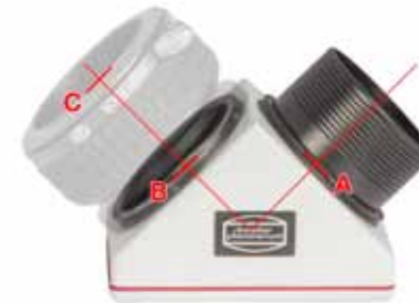
The required backfocus can be reduced from 112 mm with the ClickLock (A-C) to approximately 71,5 mm without the ClickLock (A-B).
