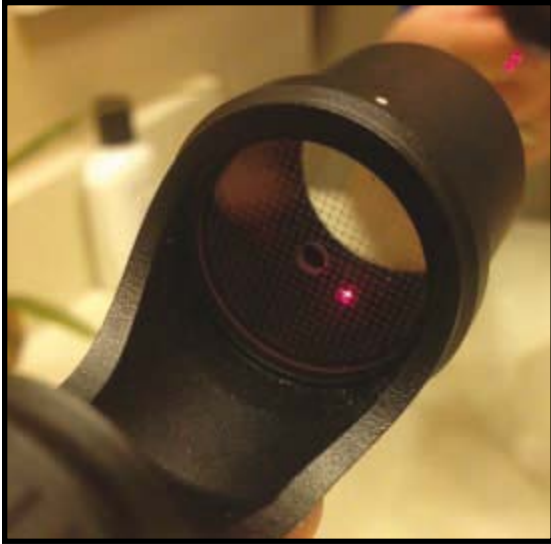
Image 10 - Etched screen of the Baader Laser Colli III.
