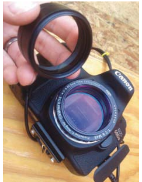
Image 2 - Baader MPCC Mark III in hand; Protective T-Ring with UV/IR Filter on the Canon 60Da.
