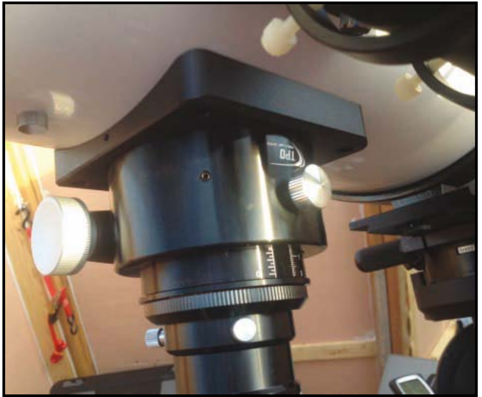
Image 7 - The 10-inch TPO Imaging Newtonian sports a 3.3-inch Crayford-style focuser. It's a dual-speed version, with a 10:1 micro-focusing dial to make perfect focus a breeze.
