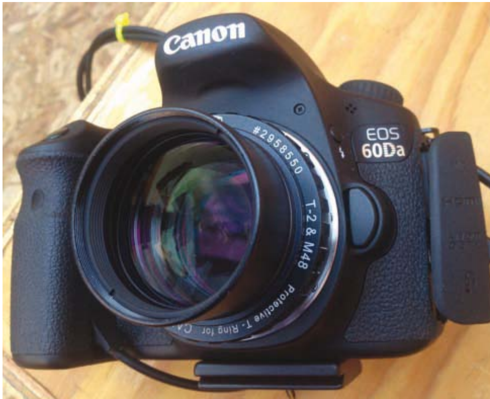
Image 3 - Baader Protective T-Ring and MPCC mounted on the Canon 60Da, ready for imaging.
