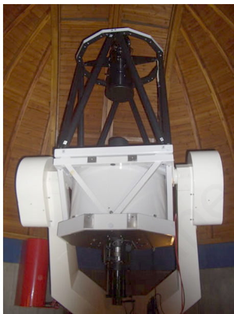
Figure 2.16: The 50 cm Cassegrain-telescope on the roof of the AIfA.
