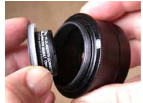
Mounting a Glasspath Compensator into the optional T2 (#16) 2"-adapter (without star diagonal) requires the white spacer ring to be placed over the thread of the GC. This way, the GC will be centered in the nosepiece.
