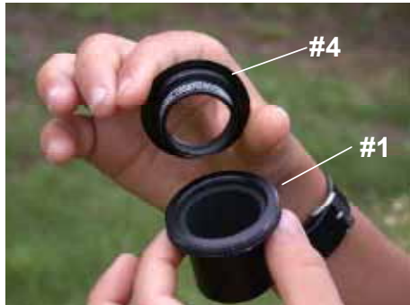
The Baader glasspath compensators (GC) #4A/B/C can be combined with many Baader-T2-accessories. For straight viewing with a 1¼" nosepiece, the 1.25x and 1.7x GCs have to be screwed into the nosepiece.
