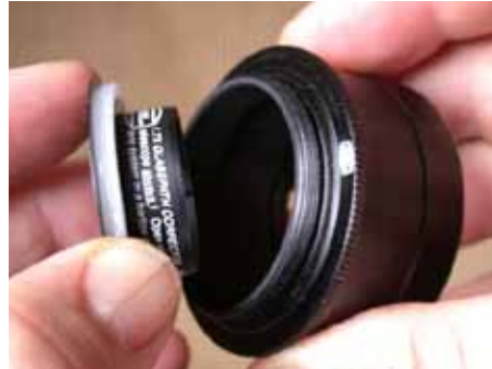
Placing the 1.25x or 1.7x GC into the optional T2 (#16) 2"-adapter (without star diagonal). The white spacer ring has to be put over the thread of the GC, so that it is centered in the 2" nosepiece.
