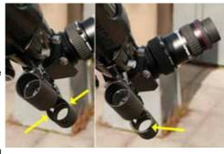
the rear barrel. On the right is the sight when the sun is not centered and the shadow only cuts the rear ring (yellow arrow). You may need to re-adjust the viewfinder for solar observation, or mark the intersections of the shadow on the rear section. Please follow the safety instructions of your telescope when you observe the Sun. You can find safe solar filters on http://astrosolar.com.
