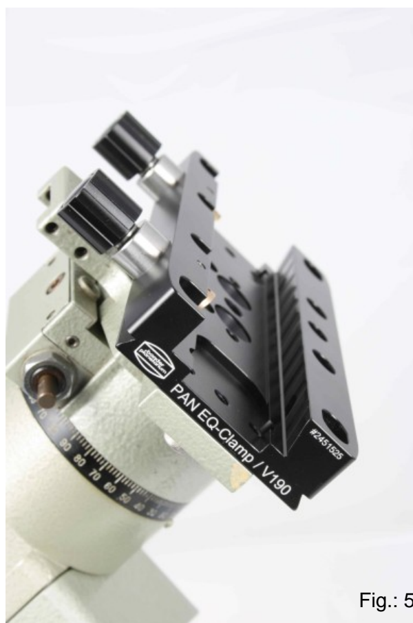
The rib milling of the PAN EQ clamp 190 multiplies the contact pressure of the two brass thrust clamps.
