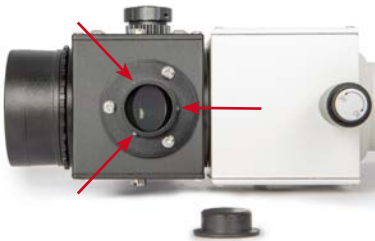
The adapter flange at the lower plate. The red arrows mark the locking screw for a pick-up prism. Loosen the larger hex screws to remove the flange, e.g. to adapt a calibration lamp. You can also see the masked mirror inside of the BFM II.
