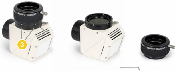
Open the six screws ③ with the 1,3 mm allen wrench, to remove the eyepiece clamp and to install e. g. a polarising filter from the top in the rotatable filter holder.
