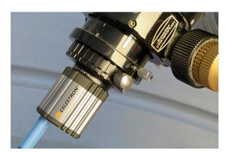
I currently use the <u>Celestron SkyRis 445 M</u> <u>camera</u> with a pixel size of 3.75 microns for monochrome lunar and planetary video sequences. The control software ICap is almost intuitive to use and runs extremely stable.
