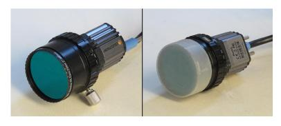
by an adapter from 2" to  $1\frac{1}{4}$ ". On the telescope side the 2" UV / IR blocking filter or the 2" IR pass filter is screwed in. The video module is then connected via a  $1\frac{1}{4}$ " socket with C-Mount thread realized. I make sure that ALWAYS a filter is screwed into the adapter. This protects the recording chip from dust, which - once it is on the chip - is very difficult to remove. That's why I always leave the camera, adapter and filter as a complete unit together.
