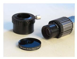
The filter even allows - if the sky is very transparent and the optics is clean - moon shots in high sun daylight. This can be helpful if you want to record special lighting situations of specific lunar structures (for example, shadows of crater walls or crater central mountains).
