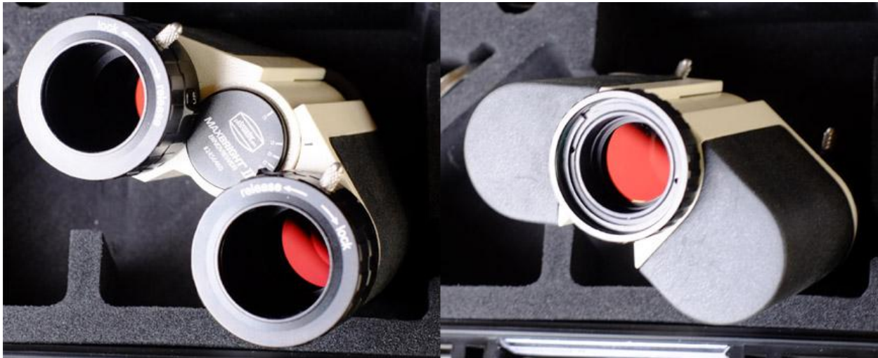
Fig 7: Eyepiece-side (left) and Telescope-Side (right) views. Note the reflex color of the prism -- a result of their designed optimization for highest transmission where the human eye is most sensitive (green light). Image Credit: Author.
