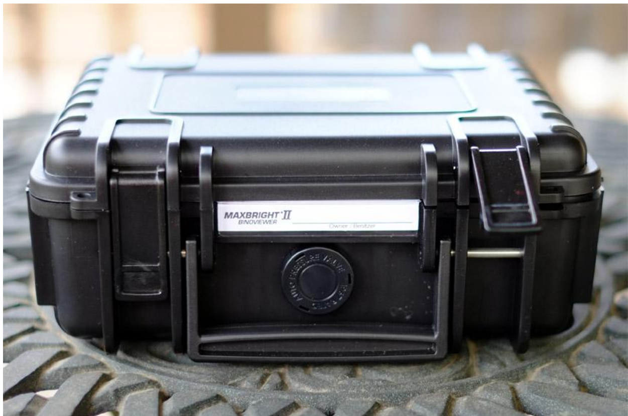
Fig 3: MaxBright II Binoviewer Hard-Shelled ABS Case (included). Note the metal pins used to hold the carry handle and secure the latches, clear plastic covered name plate for owner name/info, eyelets next to the latches for a small padlock, and the auto pressure adjustment valve on front to maintain equalized pressure between the inside and outside of the case during travel.
