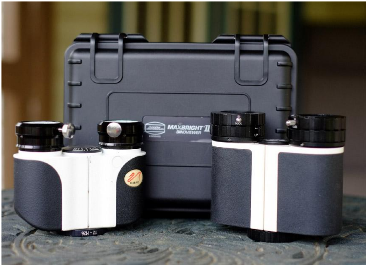
Fig 10: Size comparison between the William Optics (left) and Baader MaxBright II (right) Binoviewers. Note that the William Optics Binoviewer has its 1.25" nosepiece removed and replaced with a generic after-market T2-M26 connector allowing it to be direct connected to the Baader 1.25" T2 Prism Diagonal. Image Credit: Author.
