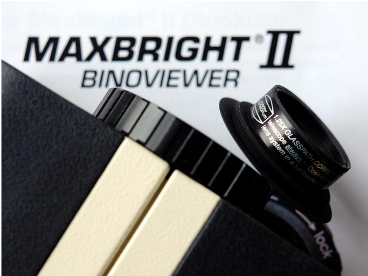
Fig 9: Baader 1.25x Glass Path Corrector (GPC) which can be inserted into the T2 Cap Nut on the telescope-end of the binoviewer (pictured). When a 2" nosepiece is then screwed into the T2 Cap Nut then GPC is held in place by the nosepiece contacting the flat place on the end of the GPC. If a 1.25" nosepiece is used then the GPC is screwed into the top of the 1.25" nosepiece prior to the nosepiece being screwed into the T2 Cap Nut. If the Baader 1.25" T2 Prism diagonal is direct connected to the T2 Cap Nut then the GPC is first screwed into the top of the diagonal.
