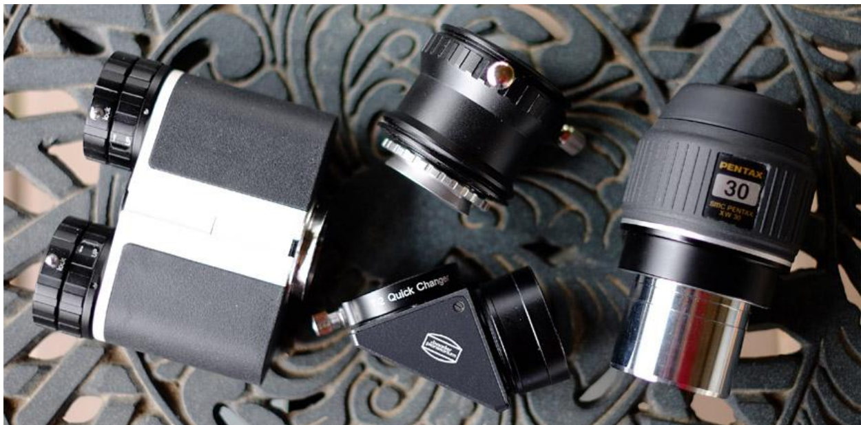
Fig 18: Baader MaxBright II Binoviewer configured with included Zeiss Micro Bayonet (left), 2" eyepiece holder with Baader T-2 Quick Change Ring # T2-07 2456320 (top center), Baader Zeiss T2 1.25" Prism Diagonal with Baader Heavy Duty T-2 Quick Changer #2456313A (bottom center), and Pentax 30mm XW eyepiece (right). Image Credit: Author.
