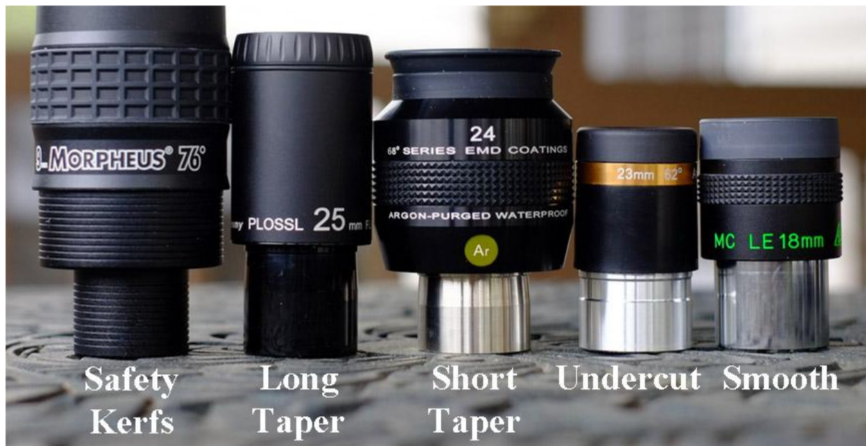
Fig 17: Barrel types tested for proper seating/alignment with the MaxBright II ClickLock eyepiece holders. Image Credit: Author.
