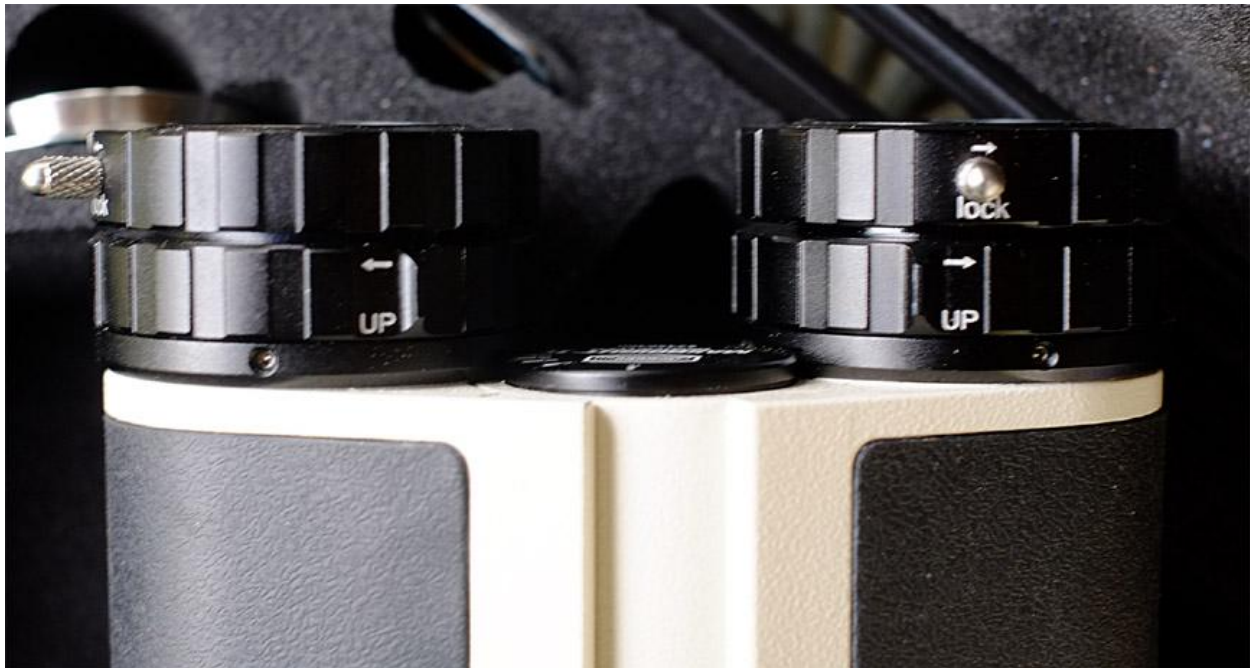
Fig 8: MaxBright II eyepiece holders with ClickLock (top) and Diopter adjustment (bottom) mechanisms. Image Credit: Author.
