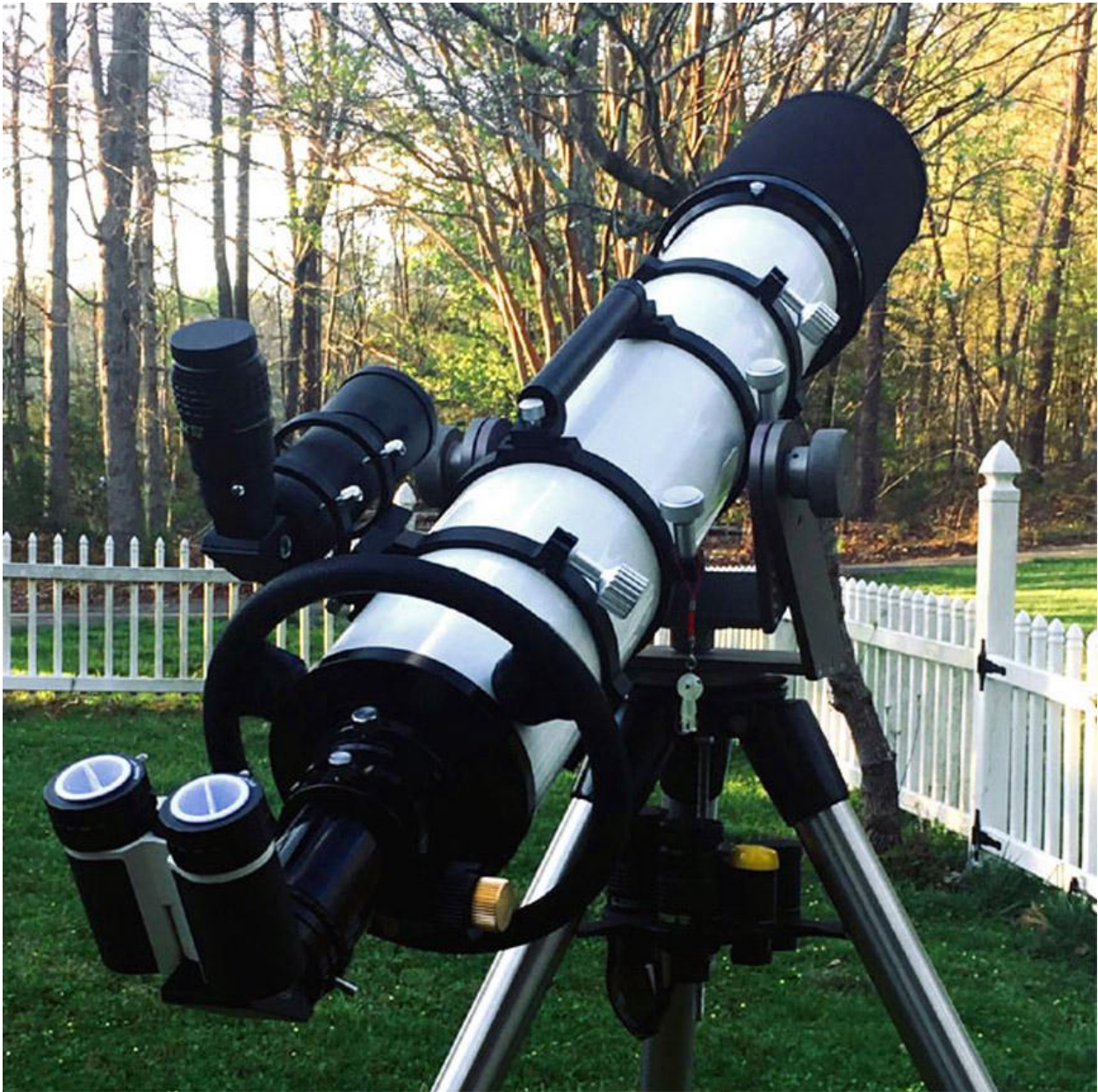
Fig 11: The MaxBright II Binoviewer connected to a Baader 1.25" Zeiss Prism Diagonal on a Lunt-152 ED Doublet f/7.9 Apo. Not pictured is a Takahashi TSA-102 f/8 Apo which was also used during the field testing. Image Credit: Author.
