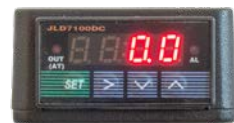
The display shows the temperature difference to the ideal operating temperature. Above shortly after powering up, below once the operating temperature is reached
