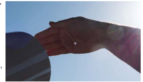
The concentrated, reflected solar radiation in front of an 80 mm telescope without D-ERF in front of the objective.
