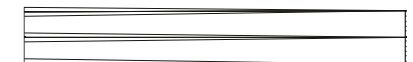
Light beam of a 6" lens telescope, which was extended to f/30 with a telecentric system
