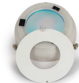
A D-ERF can be stopped down with a simple baffle
