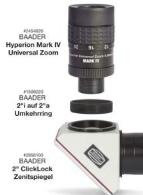
The Hyperion Mark IV Universal Zoom Eyepiece can be attached directly to a star diagonal with a 2" inverter ring #1508020
