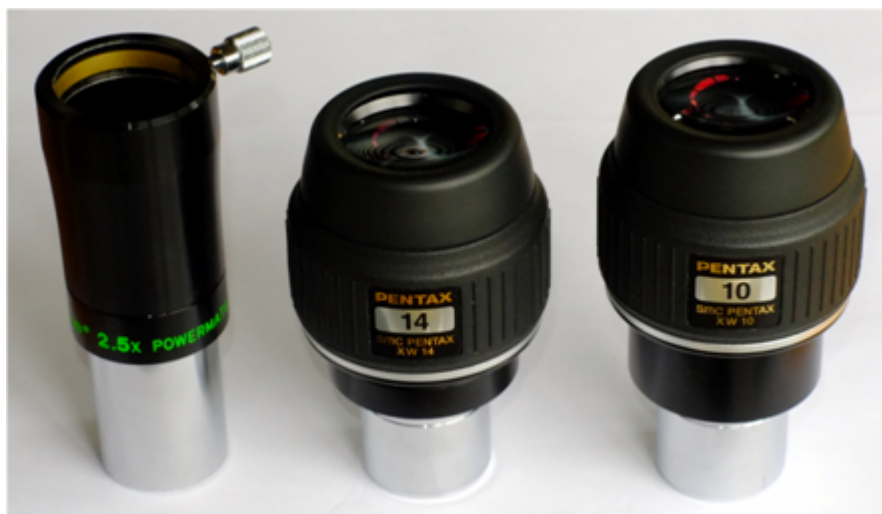
Fig 1: Eyepieces used for the test: Tele Vue 2.5x Powermate, Pentax 14mm XW, and Pentax 10mm XW.
