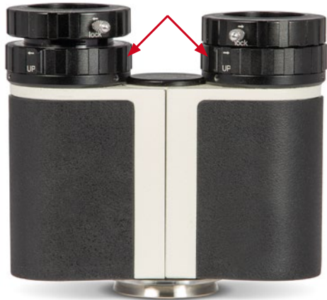
The lower ring collar is used for the diopter adjustment – compare the position of the eyepiece clamp on the left and on the right.
