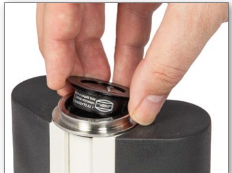
The two 1,25x and 1,7x glasspath correctors are mounted into the dovetail at the binoviewer
