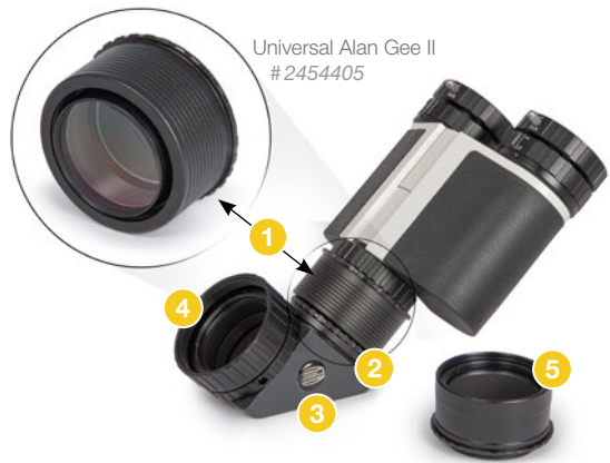
The Universal Alan Gee II 1 is connected with the help of the included 7,5mm extension ring 2 onto the T-2 star diagonal 3. The star diagonal is attached to the telescope either through the BTA-adapter for Schmidt-Cassegrains #2408160 4 or a 2"/T-2 nose piece #2408150 5.
