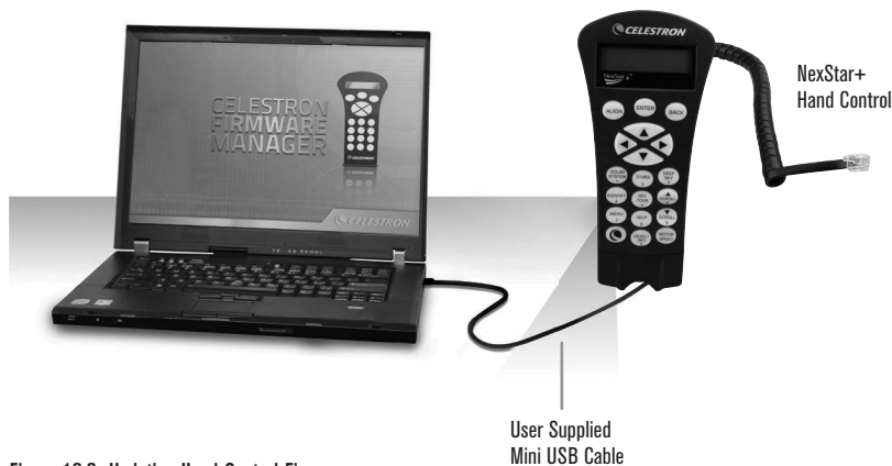
Figure 12.2 Updating Hand Control Firmware
