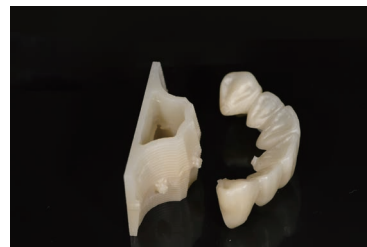
Support removal finished
