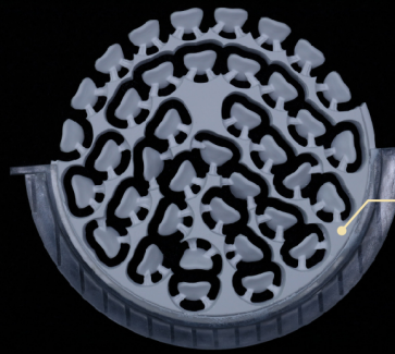
One disc of zirconia milling 38 veneers.
