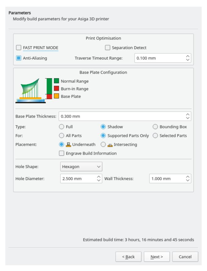
A "base plate" is an area to be printed directly on the platform. This is required when building parts with support structures as it helps bond the supports to the build plate. The base plate can also ease the task to remove the build from the platform after the printing is finished.
