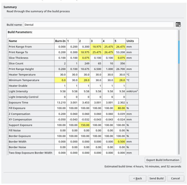
The date/time toggle button to the right of "Build name" allows you to choose whether to set the build name to the current date/time by default (e.g. 20180316-1632).
