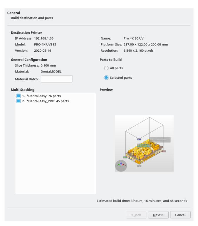
If the last checked build has a multi stacking scaffold, it will not be included as it is not necessary. Clicking "Next" will validate the parts to build and warn you of any potential problems.
