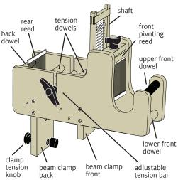
FIGURE 3: TENSION BOX PARTS
