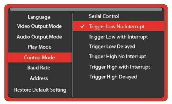
**Serial Control** is to use a Hydra<sup>®</sup> input expander or external show control device or micro controller like a PIC, Atmel, Arduino, Raspberry Pi, or etc. using serial communications.
