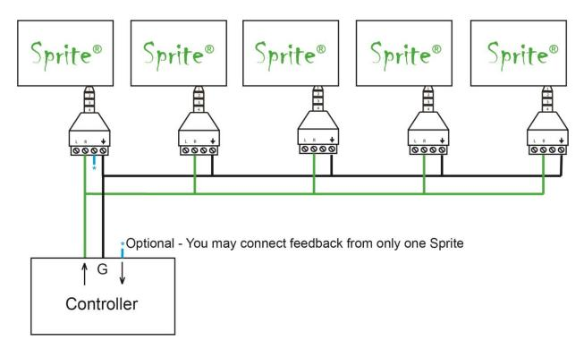
Limitations on the number of Sprites on the bus include length of wire, type of wire and baud rate. Low capacitance wire and lower baud rates will allow longer distances and / or more Sprites on the bus.
