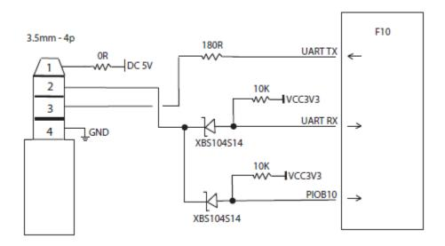
The Sprite is designed to work with 3 to 5 Volt TTL level serial data.
