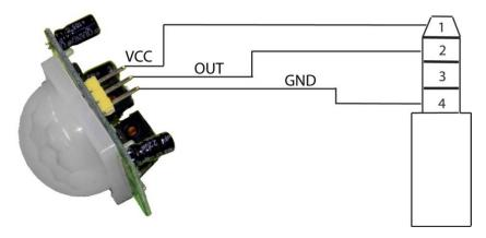
Wiring a 5 Volt motion sensor
