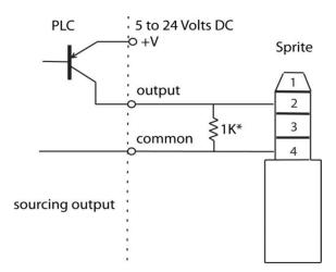
The Sprite® has an internal 10K pullup so the Sourcing output requires a low resistance from Output to Common to pull the Sprite's internal voltage down to a "LOW". The 1K\* shown is an example and can vary depending on the +V voltage. Consider the Watt rating of the resistor.
