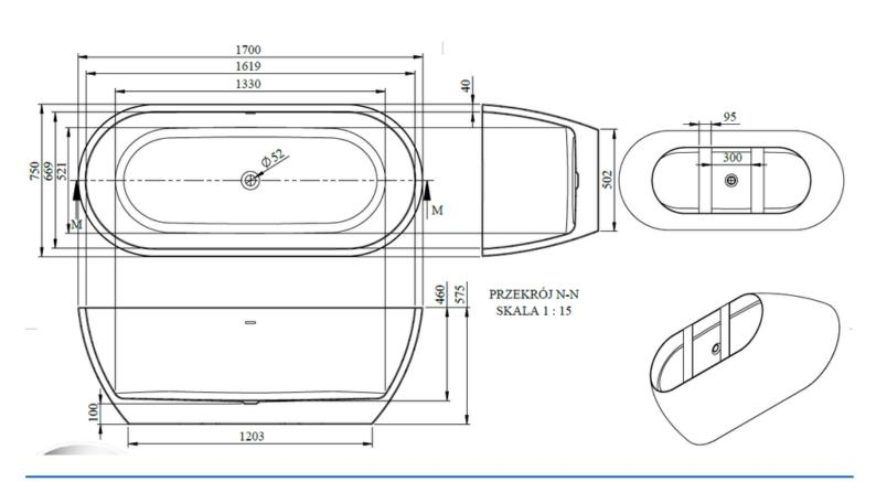
All measurements shown are in millimetres. Drawing sizes are not to scale. Measurement accuracy ±5mm. Halo Tiles & Bathrooms reserves the right to make changes and/or modifications to products and specifications without prior notice
