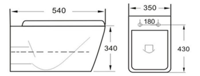
All measurements shown are in millimetres. Drawing sizes are not to scale. Measurement accuracy ±5mm. Halo Tiles & Bathrooms reserves the right to make changes and/or modifications to products and specifications without prior notice
