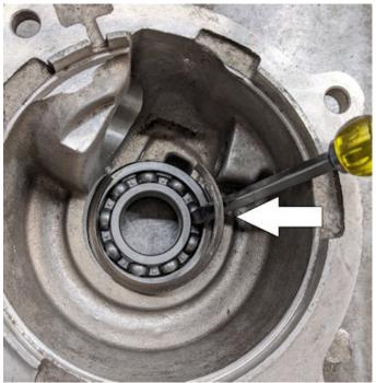
After ensuring the bearing and retaining ring are both properly installed you may need to press the seal into the housing.
