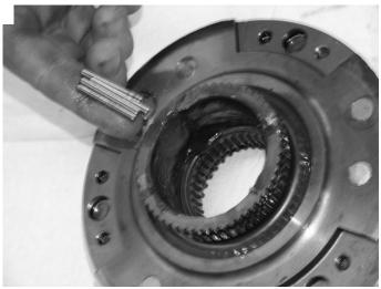
After removing the intermediate sleeve, the snap-ring which retains the planetary assembly to the main-shaft will be accessible. Remove this snap ring, then slide the planetary assembly off the main-shaft.
