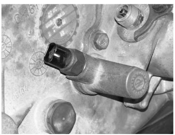
Confirm your transfer case is a 242 with identifying tag. Check to ensure that the stock output shaft has 27 splines, by counting the splines. Please also check that the speedometer housing appears to be correct for your application. The original housing may or may not have a port for insertion of a switch. If your old housing did not have this port you will not need it with the supplied housing and visa/ versa.
