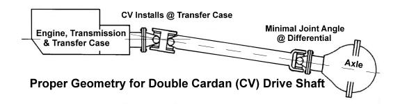
**Note:** To prevent drive shaft torsional vibrations, your net U-joint angle at the differential should be no less than 1 degree and no more than 3 degree's different than the drive shaft slope. It is best to leave the pinion lower rather than higher to allow for natural spring wrap.
