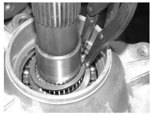
The basic process is a simple and partial dis-assembly of the transfer case and the re-assembly in a reverse order using a modified main-shaft. The transfer-case will be identical to its original configuration up to and including the rear out-put bearing. Any snap ring(s) that was originally on the main-shaft and rearward of the rear out-put bearing will be discarded.
