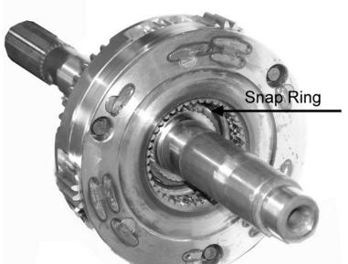
Start by removing the snap-ring on the inboard end of the main-shaft and the tabbed thrust washer which retain the intermediate sleeve onto the main-shaft. Note the orientation of this intermediate sleeve, thrust washers and other parts as they are removed as they will need to be installed onto the replacement shaft in exactly the same order.
