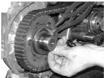
Remove the snap ring that retains the chain sprocket to the front out-put shaft.
