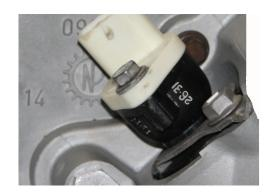
Remove the four bolts securing the speedometer housing to the rear case half. Gently pry the speedometer housing away from the rear case half.
