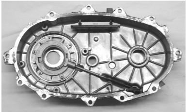
Clean all mating surfaces of the case halves and housings of all old silicon or RTV sealant and oil film. Before assembling these parts, wipe a thin film of RTV sealant across the finish machined mating surfaces.
