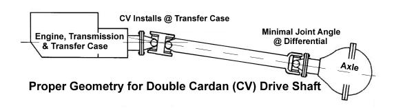
**Note:** To prevent drive shaft torsional vibrations, your net U-joint angle at the differential should be no less than 1 degree and no more than 3 degree's different than the drive shaft slope. It is best to leave the pinion lower rather than higher to allow for natural spring wrap.
