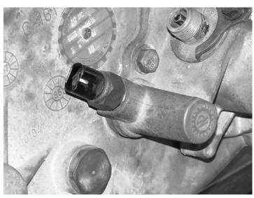
Confirm your transfer case is a 242 with identifying tag. Please also check that the speedometer housing appears to be correct for your application. The original housing may or may not have a port for insertion of a switch. If your old housing did not have this port you will not need it with the supplied housing and visa/versa.
