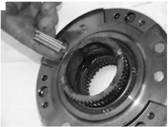
After the reassembly of the main-shaft components, wrap the chain around both sprockets and slide the main-shaft assembly back into place while simultaneously sliding the front chain sprocket onto the front out-put shaft. Secure the Front chain sprocket to the front out-put of the transfer case with the snap ring. This is reverse of the dis-assembly procedure.
