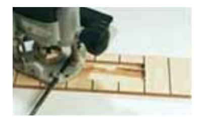
Just route-out a section on the reverse side of a plank and install the **fidbox**<sup>®</sup>.
