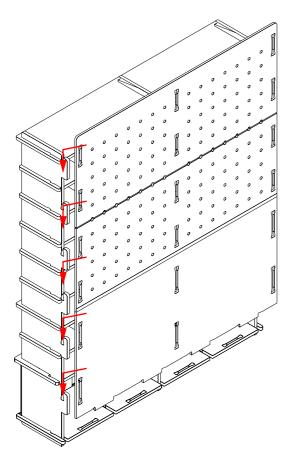
NOTE. ensure these male joins insert into corresponding female holes on bottom piece
