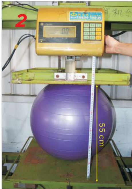
Inflate the Fitness ball to indicate size 55cm, Put ball in testing machine.
