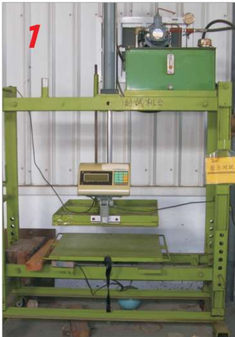
Pressure Testing Machine
