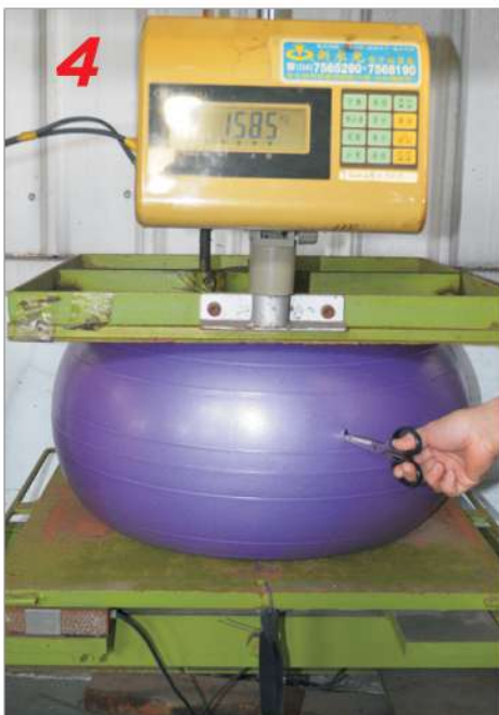
Punch the ball with 5mm-10mm wide blade, the ball leakage slowly not burst as attach picture
