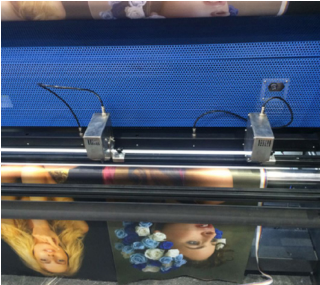
Figure 1: Hot Knife function for automatic trimming.
