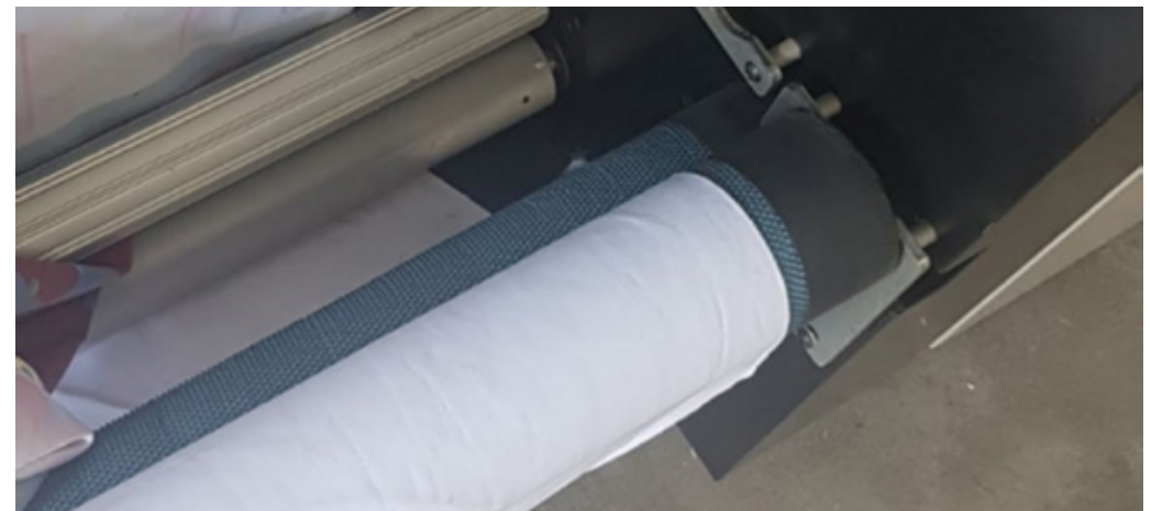
Figure 3: Roll to floor pinch rollers option.
