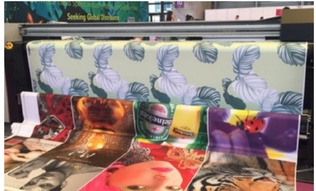
Figure 2: Roll to floor Free fall media option.
