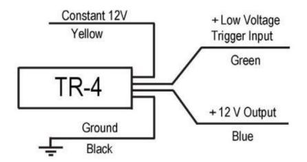
Connect the Green wire to the DSR1 remote out wire (blue/white) and the blue wire of the TR4 to the amplifier(s) remote input wire. Tag positive and ground (yellow & black) directly from the DSR1 power black and yellow power wires. Be sure to fuse the yellow wire if you are getting power for the DSR1.
