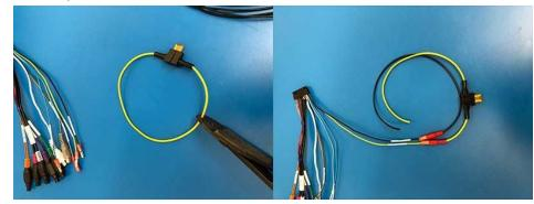
Above shows how to connect a standard fuse holder.
