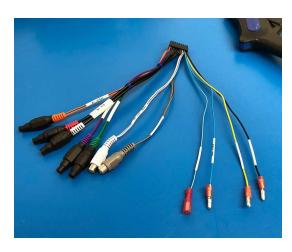
A typical installation will only require that the front RCA inputs are used. Heat shrink or tape off the ends of the remaining RCAs (Digital in, Aux, & Rear Input). We recommend that you use bullet type connectors on the remaining 4 wires. The industry standard for all connectors is that a circuit supplying power or signal uses a female connector and a circuit that receives power or signal uses a male connector. This is to avoid electrical shorts when the connectors are not together.
