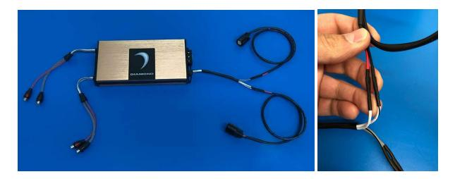
Use the harnesses that came with your plug and play signal harness labeled "Speaker Pod Harnesses". On amplifiers that have wired speaker outputs these harnesses you will need to do wire to wire connections. The female Molex connectors will plug directly into your speaker pods in the fairing. It doesn't get much easier than that!
