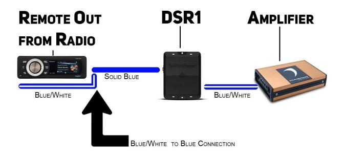
Notice the connection point between the radio's blue/white wire and the DSR1 solid blue wire. Most radios will have a Blue/white wire. Never connect the radios Blue/white wire to the DSR1 blue/white wire. This will destroy the power supply of the DSR1 and potentially the radio. This is not covered under warranty.
