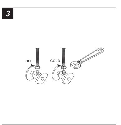
3.Connect the flexible hose to water supply valve (not included), and tighten it with adjustable wrench. **DON'T OVER TIGHTEN!**
