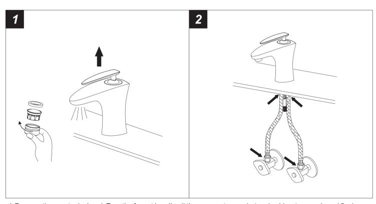
1. Remove the aerator by hand. Turn the faucet handle all the way on, turn on hot and cold water supply and flush water lines for one minute. Reinstall aerator by hand. 2. Check all connections at arrows for leaks, re-tighten it if necessary. BUT DON'T OVERTIGHTEN!
