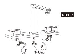
Connect and tighten the T-Joint to the shank.
