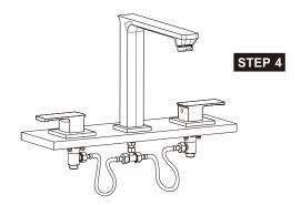
Connect hoses from valve body to the T-Joint .
