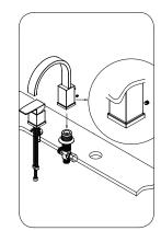
Unscrew the Allen screw in back of the spout. Pull apart the spout from its connector (do not unscrew). Separate the spout flange from the spout. Place o-ring underneath the spout flange and place the flange over the center hole between the handle and hand shower.
