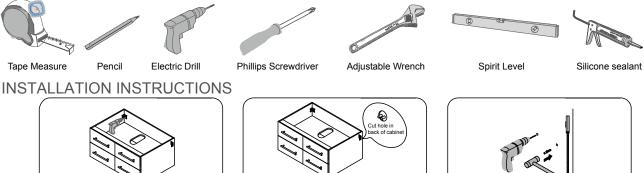
① Drill holes to match stud placement in wall.
