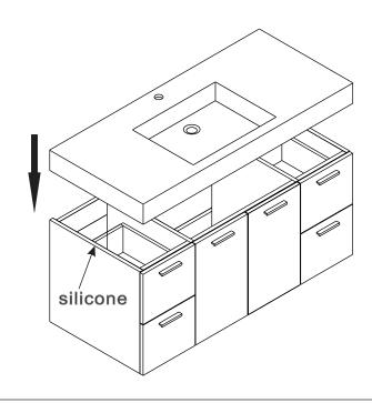
6 Licensed professional installation is recommended. These instructions are for mounting into studs or other in-wall reinforcement, drywall alone is not sufficient to support wall-hung vanities. Other installation techniques may require a licensed professional.
